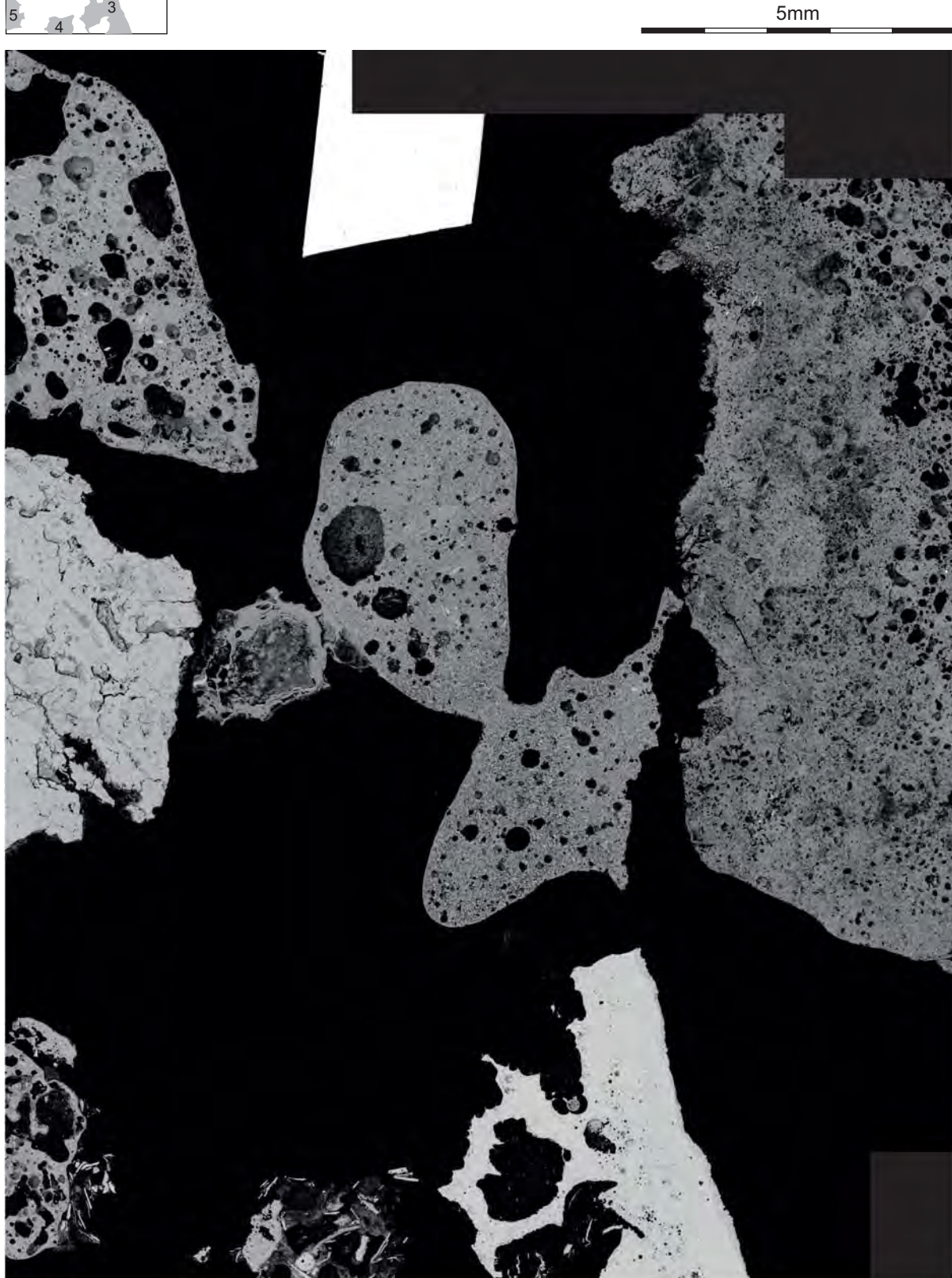
Plate A1: Sample HGA1. Tabular microresidues. Backscattered electron image montage of central part of mount with key to particles.
