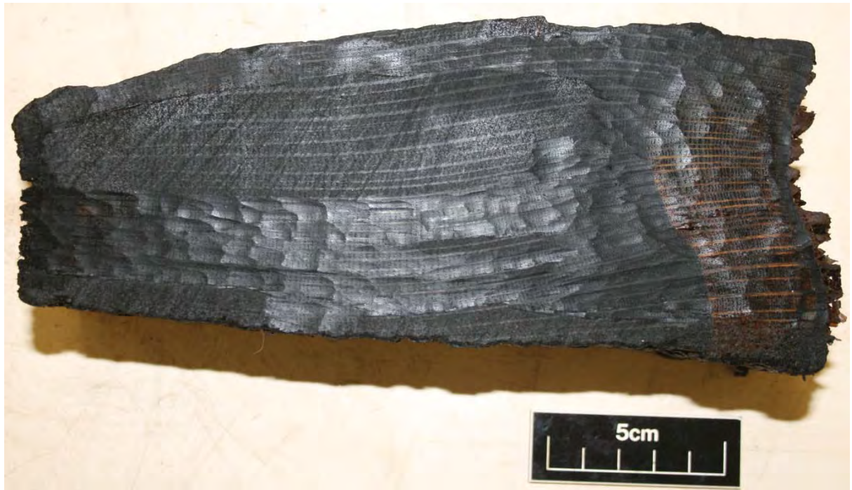
Figure 12.111 photograph of dendro sample 2 from sample 49, showing included sapwood on lower right of sample and heartwood/sapwood boundary
