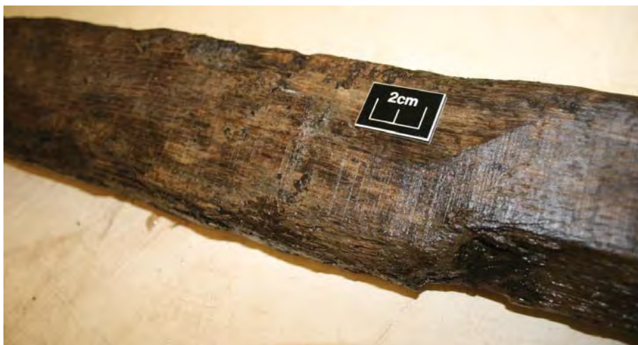
Figure 12.60 photograph of vertical saw marks on upper face of sample 52 4 of 4
