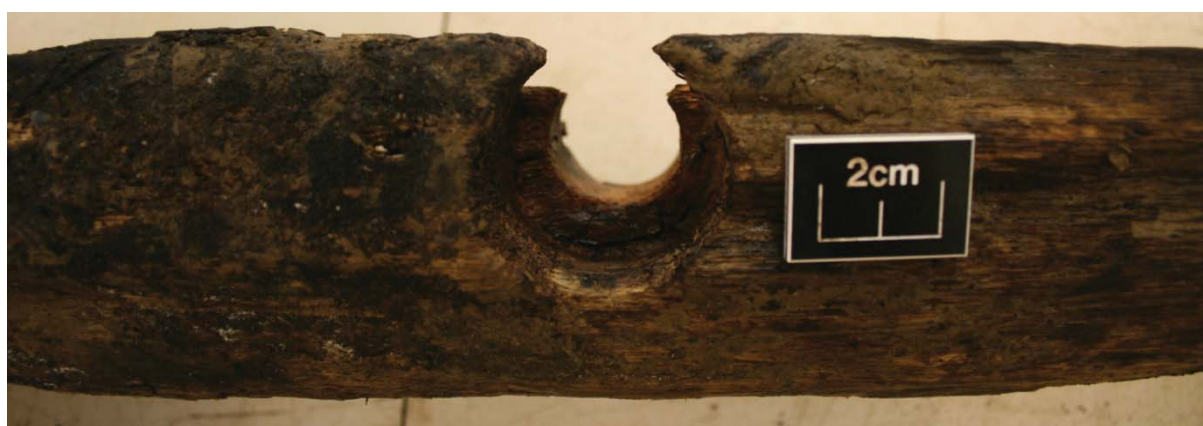
Figure 12.66 photograph of peg hole on sample 53 1 of 4
