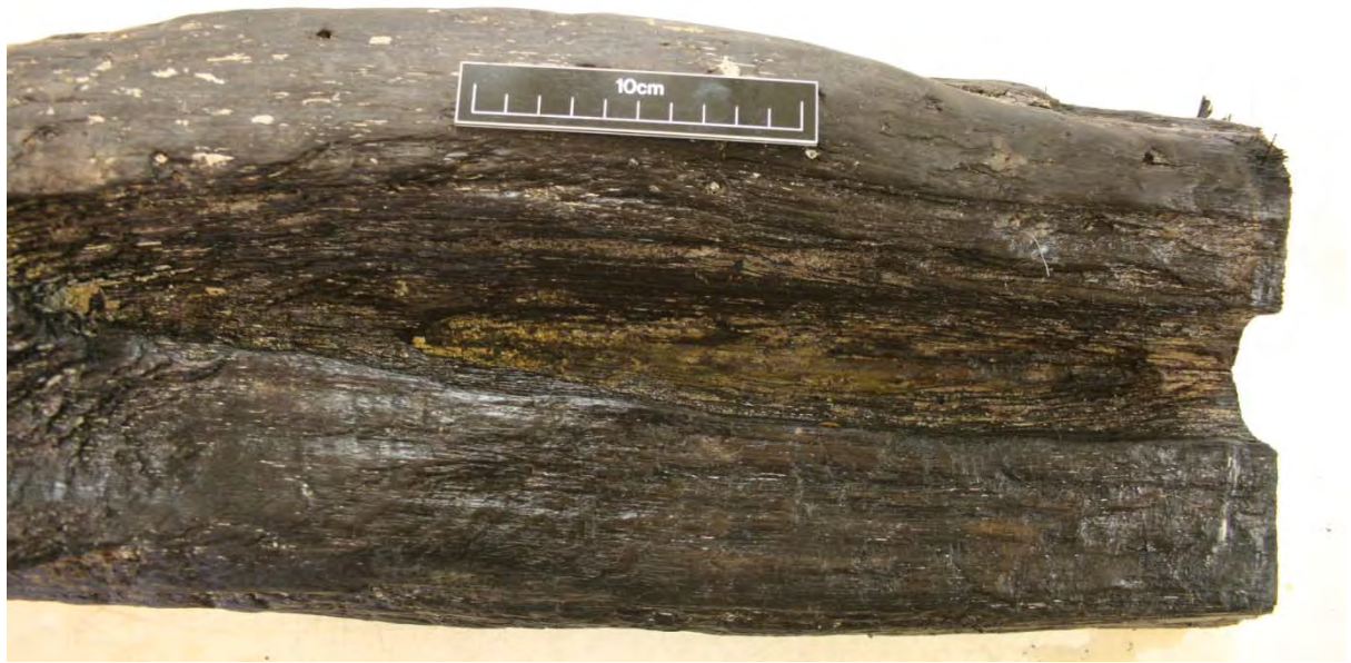
Figure 12.95 photograph of sample 58 2 of 2 showing eroded heartwood
