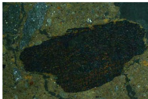
Fig. 14.17: As Fig 16, under OIL; note ochreous orange iron (lepidocrocite – \text{FeO}(\text{OH}) ?) staining of fine soil.
